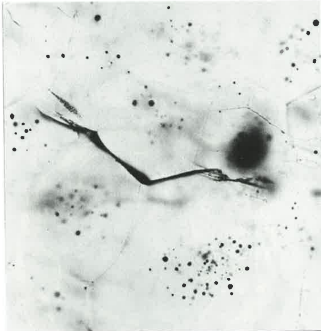
Fig. 9.10. Spontaneous microcracking associated with thermal expansion anisotropy stresses in alumina. Initiation occurs at tensile grain facets, arrest at compressive facets. Note small pores within individual grains. Transmitted light. Width of field 125 \mu\text{m} . (Courtesy P. Chantikul & S. J. Bennison.)
